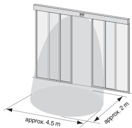
Installation height 2200 mm / angle of detection field 30°
