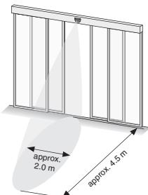
Installation height 2200 mm / angle of detection field 30°
