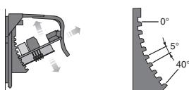
The detection field can be swivelled in 5 steps from 0 to 40°.
